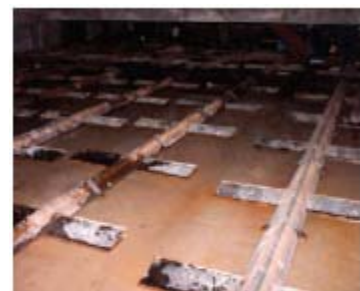
Pousoir de type «push floor» Source : Biomasscenter www.biomasscenter.org
